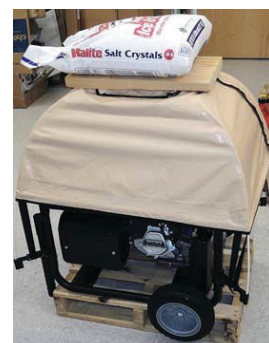
GenTent withstanding 55.5 LBS of weight, equivalent to 19" of snow
