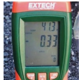
Intake vacuum with (above) and without GenTent
