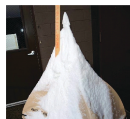
GenTent withstanding 55.5 LBS of weight, equivalent to 19" of snow
