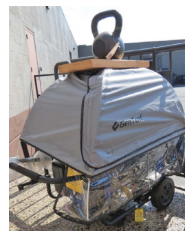
GenTent withstanding ~60 LBS of weight, equivalent to 20" of snow
