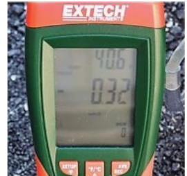
Intake vacuum with (above) and without GenTent
