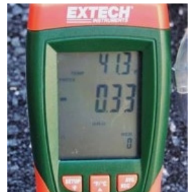
Intake vacuum with (above) and without GenTent
