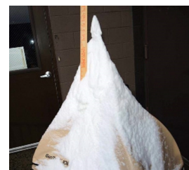
GenTent withstanding ~60 LBS of weight, equivalent to 20" of snow
