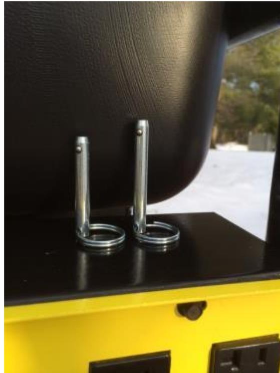
The handle is permanently connected to the frame with 4 carriage bolts. Replace these bolts with either of the quick detach pin types above by unscrewing the existing bolt and simply sliding the quick detach pin into place (then locking it with the clip pin as appropriate).
