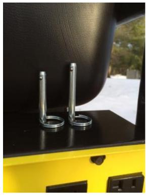
The handle is permanently connected to the frame with 4 carriage bolts. Replace these bolts with either of the quick detach pin types above by unscrewing the existing bolt and simply sliding the quick detach pin into place (then locking it with the clip pin as appropriate).
